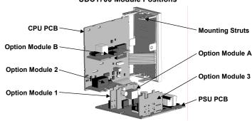
To access modules 1, A or B, first detach the PSU and CPU boards from the front by lifting first the upper, and then lower mounting struts. Gently separate the boards.
